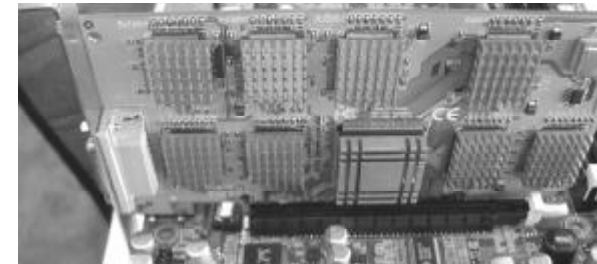
figure 2:PCI E-1X interface card insert into the PCI-E 16X slot
