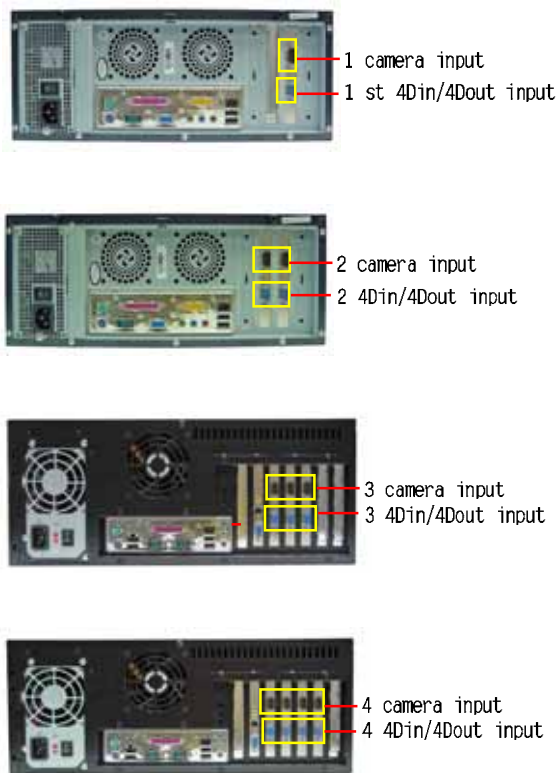
Figure 11-1: Rear View of DVR with GPIO interface
