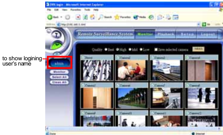
Figure 14-5: Remote Monitor Screen - Remote Monitor
